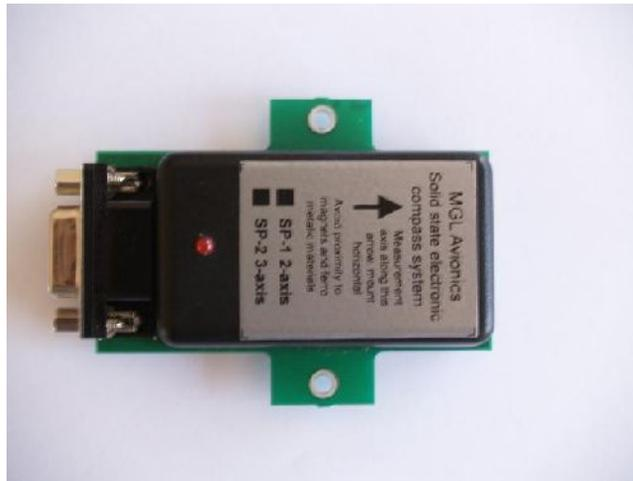
The SP-2 magnetometer is a three axis, tilt compensated electronic compass system. It outputs magnetic heading information.
