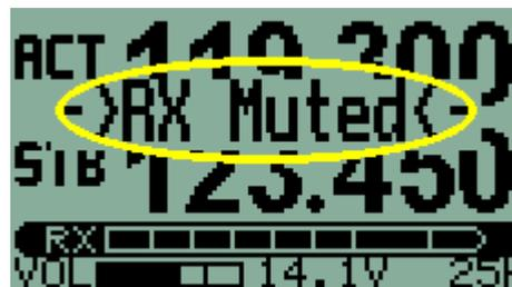
Radio volume is restored by holding the VOL/TEST knob down and rotating clockwise. Also, volume is automatically returned to normal by using the transmitter (pressing a PTT).
