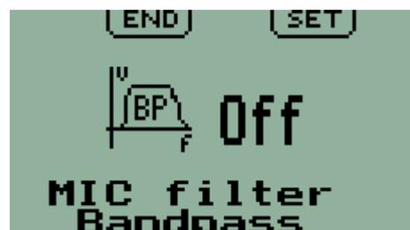
This can help reduce the effects of unwanted noise, in particular at low and high frequencies. This filter has a sharp cutoff for frequencies below 500 Hz and above 2.4KHz.
