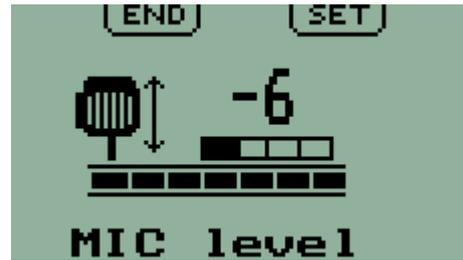
NB: For a single microphone, the level shown by the bargraph is for the Pilot microphone input ONLY. No level is shown for the passenger microphone. The adjustment affects all microphones equally.
